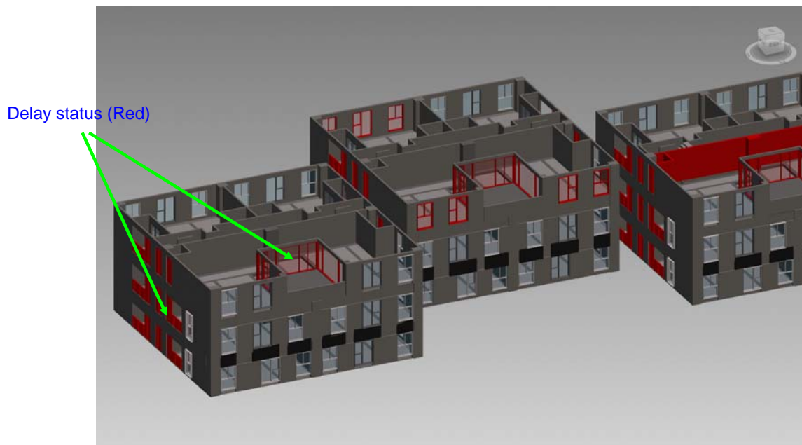
Figure 18. The alarm sample illustration of as-built updating schedule integrated with BIM model (2/2)
