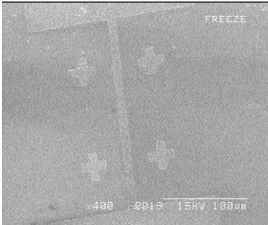
Figure 3.2.1: Optical lithography technique for the SNS device. (a) Mask. (b) Patterned EBCO thin film on STO. (c) The SEM image for the superconductor bridge is the region that circled by dotted line in (a) (b).  $W$  is the width of bridge,  $W \sim 10 \mu\text{m}$ .
