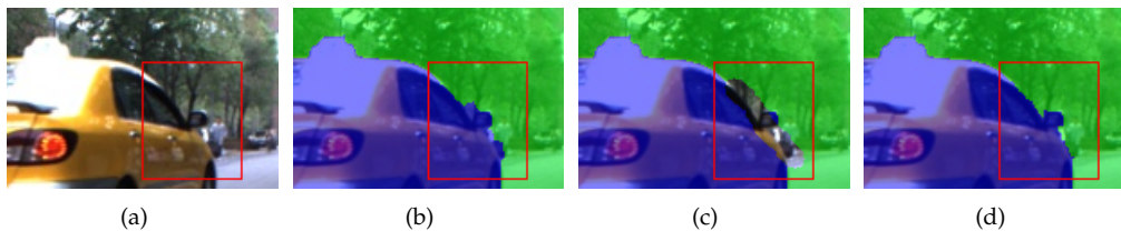
Figure 4.3. An example of clearing the improperly segmented region and apply GrowCut again. (a) The original image. (b) Improperly segmented image. (c) Clear the labels near the desired contour. (d) Apply GrowCut again.
