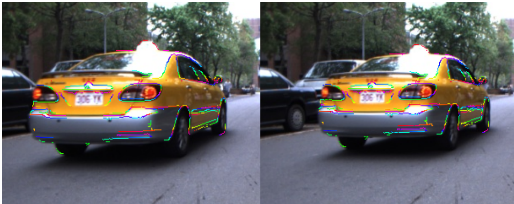
Figure 4.6. User specified points on the edge that are associated by optical flow. The corresponding points are denoted as the same color
