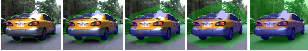
Figure 3.3. Automata evolution steps. Blue is the object label while green is the background label.
