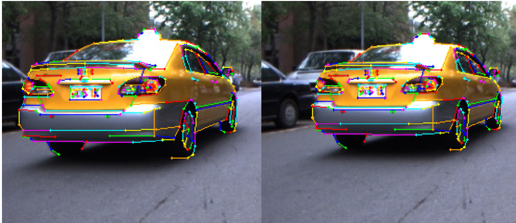
Figure 4.5. An intuitive idea of labeling salient feature correspondences. Corresponding line segments are denoted as the same color.
