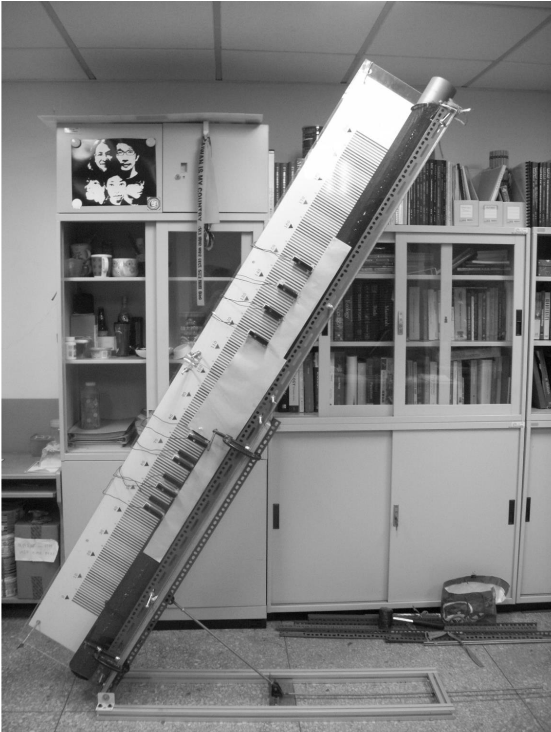
Figure 17. The contraption for measuring sprint speed of lizards
