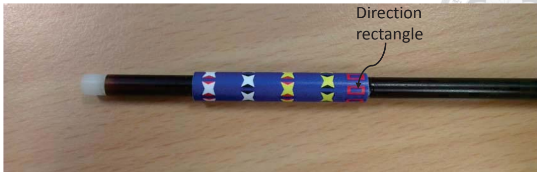
Fig. 4-14 The hollow rectangles in the right of marker set are direction rectangles, which are used to determine marker direction.
