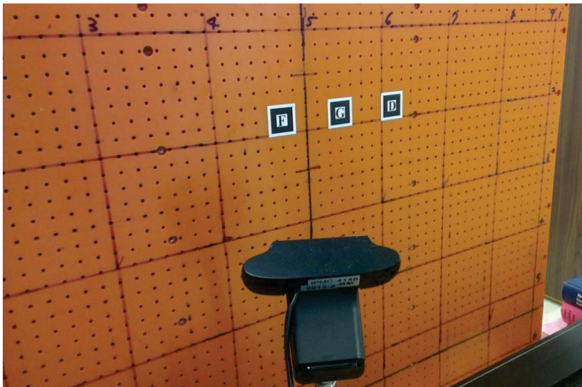
Fig. 5-2 A square marker is attached on a specific position of the panel. When camera catches image with the marker, the position of the marker in camera coordinate can be estimated.
