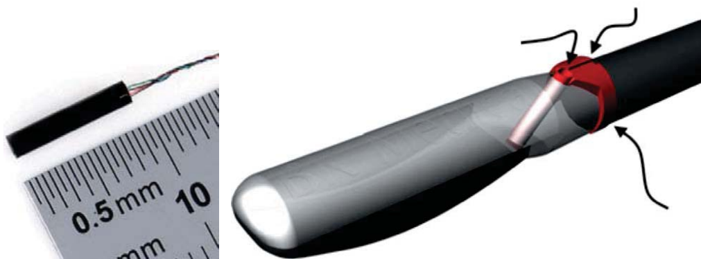
Fig. 2-6 A directional magnetic field sensor (left). A directional magnetic field sensor was inserted rigidly into the tracked target (right) [6].
