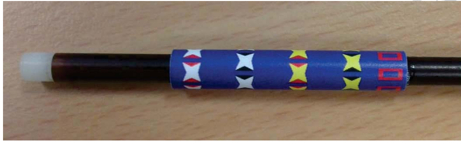
Fig. 4-12 Illustration of a marker set affixed to instrument. Markers in different layers has different color combinations, which is the same when markers are in the same layer.
