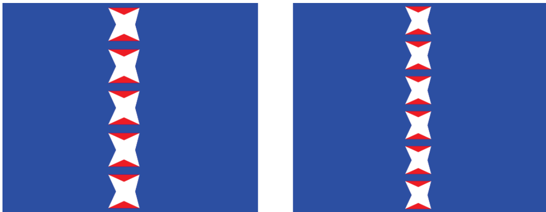
Fig. 4-18 Five markers a layer (left). To solve view-invariant problem, one method is adding number of markers on each layer (right).
