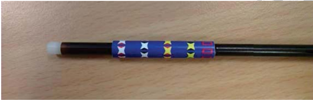
Fig. 1-4 A cylindrical marker set is affixed to a cylindrical marker module which is attached to instrument.
