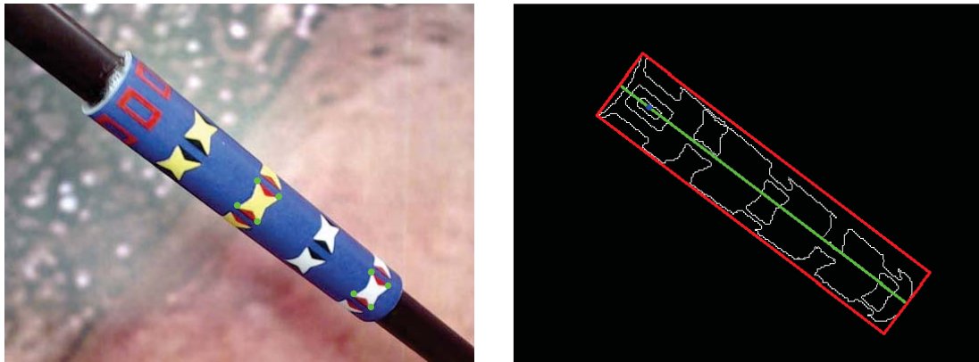
Fig. 4-22 The markers whose corner points are marked green are filtered as the confident markers used to calculate transformation matrix. The criteria to filter confident markers are distances between markers and major axis of background region.
