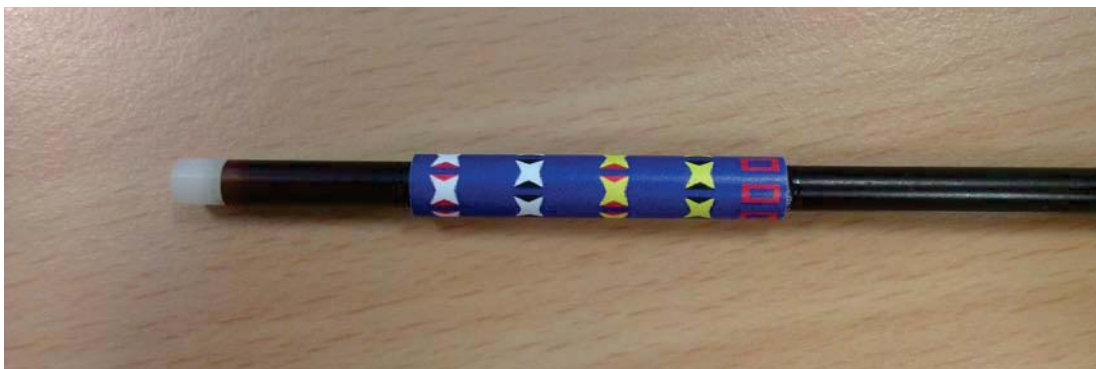
Fig. 4-6 Complete cylindrical marker set is affixed to a marker module attached to instrument.
