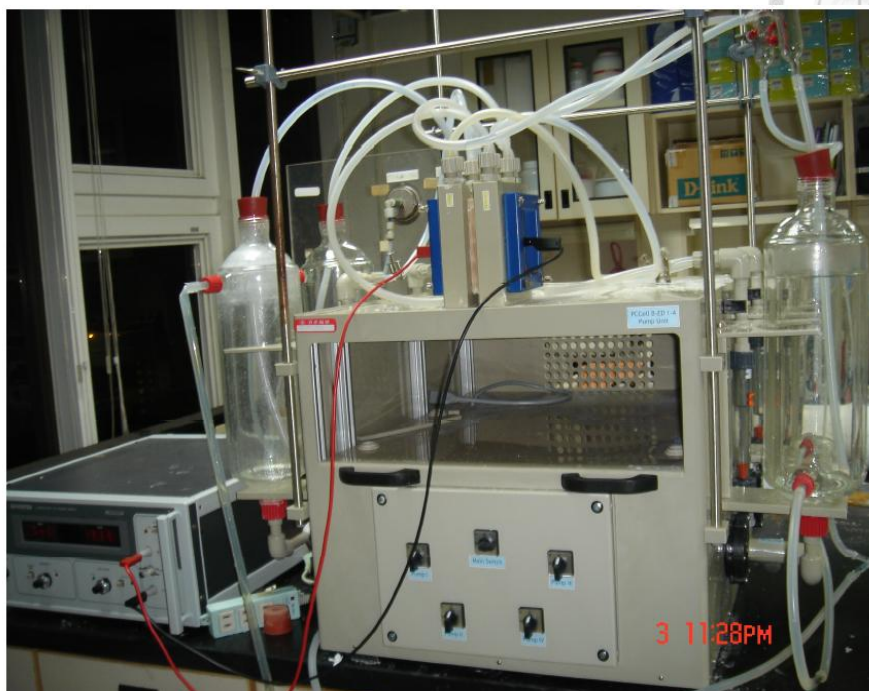
Fig.3-1 Picture of LAB-scale electro dialysis system and DC power supply.
