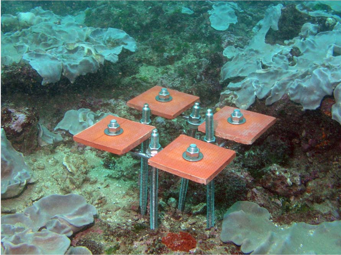
Fig. 4.2 A set of settlement plates used for coral recruitment surveys in this study.
