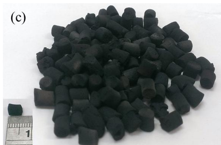
Fig. 4.2 Appearance of the support and synthesized catalysts in granule.
