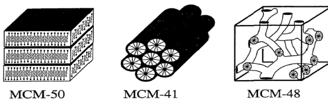
Fig. 2.8 Schematic diagram of the M41S materials, MCM-50 (layered), MCM-41 (hexagonal) and MCM-48 (Cubic).(Tangestaninejad et al., 2009)
