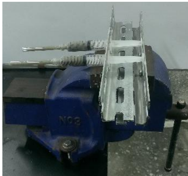
Fig. 3.5 Homemade extruder for the granulation of SBA-15 p .
