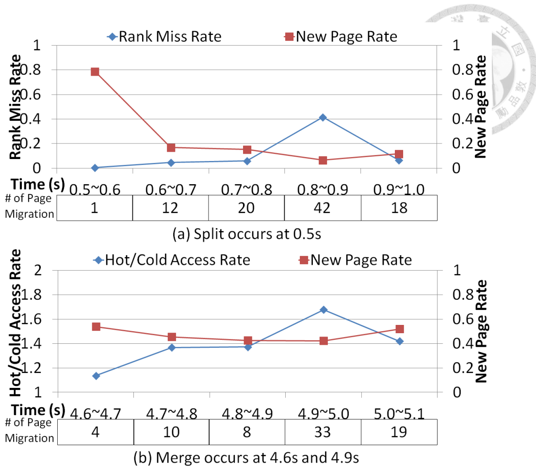
Figure 4.13: Rank Miss Rate, Hot/Cold Access Rate, New Page Rate and the number of page migrations for SPEC2000-1 with the dynamic BW estimation method in 0.5s~1.0s and 4.6s~5.1s for evaluations to Deferred Page Migration.
