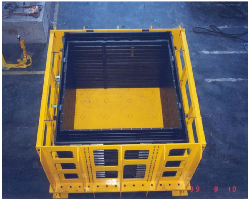
Figure 2-15 Picture of the empty laminar shear box. (After Ueng et al, 2006)
