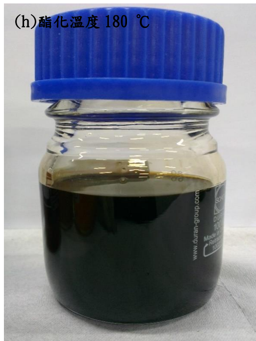
Fig. 4.13 Color difference of the oil after the esterification reaction carried out at different temperatures.
