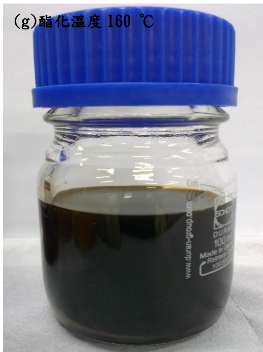
Fig. 4.13 Color difference of the oil after the esterification reaction carried out at different temperatures.
