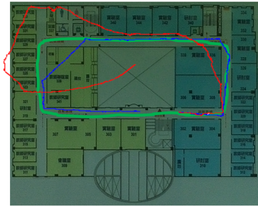
Figure 4.6: Estimated results of long-term round trip. The red trajectory is the visual alone result, the blue trajectory is the fusion result and the green trajectory is the ground truth. The total distance of blue and red path are 142.9 m and 116.3 m, respectively. The manually measured ground truth is 119.7 m.
