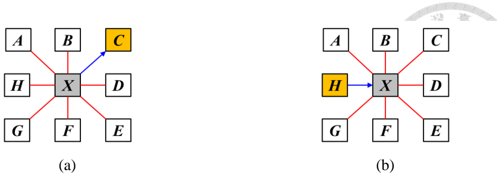
Figure 4.4: The two-way propagation policy. (a) the first-propagation direction. (b) the second-propagation direction.
