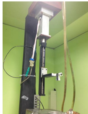
Fig. 2-9 The feeding system used to control the holder to slowly travel to provide more materials for fiber drawing: (a) control panel, (b) a silica tube holder.
