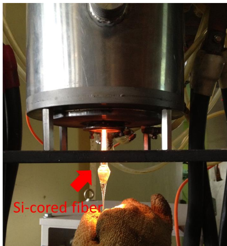
Fig. 2-13 The tube is molded into a Si-cored fiber by drawing.
