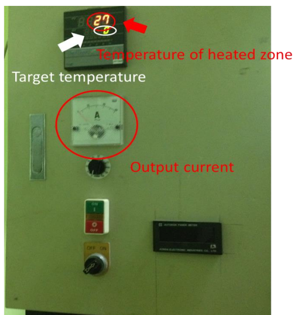
Fig. 2-11 The heating control panel, which controls output current to the heating resistors and monitor the temperature of heated zone.
