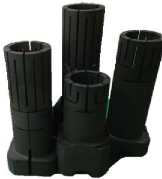
Fig. 2-8 Manufactured graphites tube served as a heating source.
