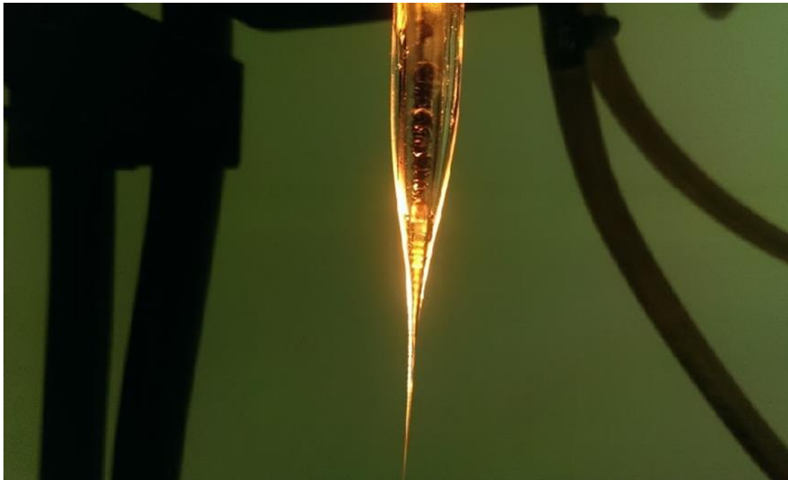
Fig. 2-4 A fiber preform in tapered shape with strong light emission just coming out from the furnace.
