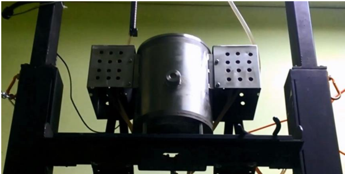
Fig. 2-2 A front view of the homemade drawing tower.
