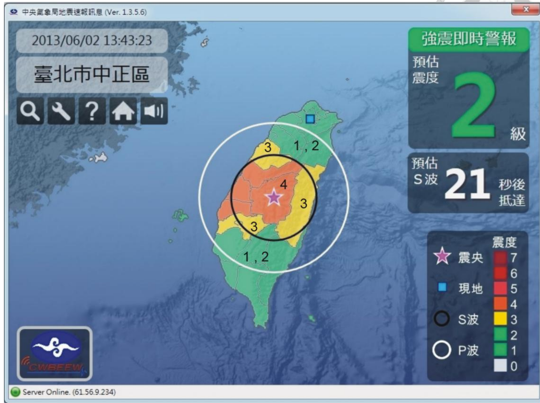
Figure 3-10. Graphical output of the eBEAR system during a simulation of the M_L 6.5 earthquake in central Taiwan. (top-left) The origin event time and the name of the target city. (center) The rectangle represents the target area. The black line represents the wave front of the P wave. The white line represents the wave front of the S wave. (center-right) The countdown timer for S-wave arrival. (top-right) The predicted intensity of the target area.
