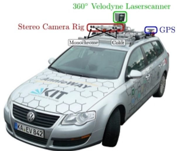
FIGURE 6.11. Autonomous platform AnnieWay that was used to capture KITTI dataset. Image from [26]
