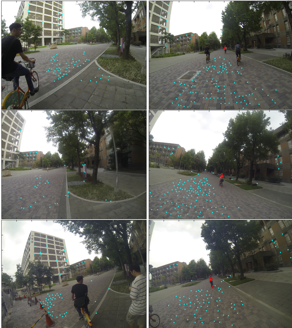
FIGURE 6.20. Left row are images from the 3 cameras taken at f=1 , right at f=225 . Blue points are static features, red features that are moving.
