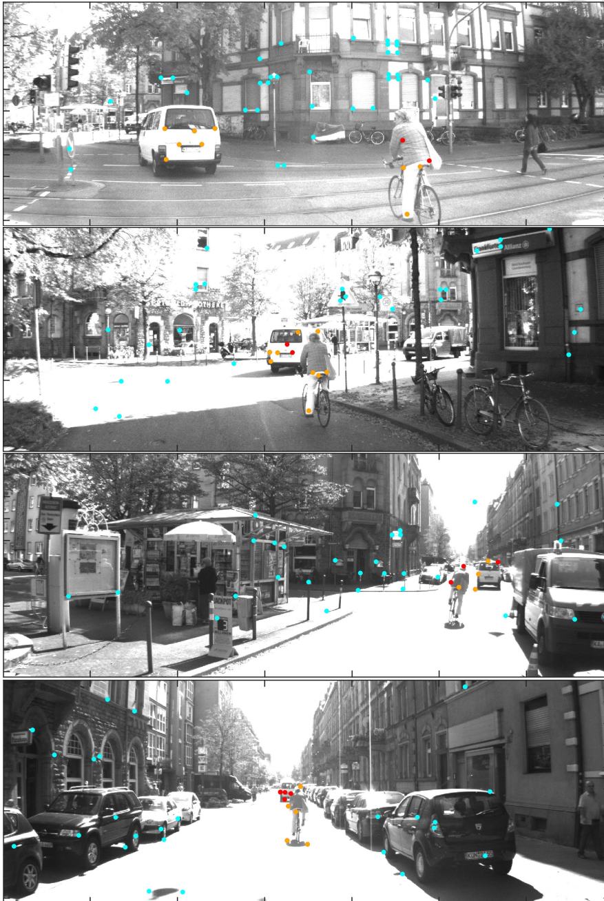
FIGURE 6.12. Frames 1, 52, 104 and 158 from the used KITTI image sequence. Blue points are static features, orange and red features that are moving. Orange points are features that are visible in both cameras.
