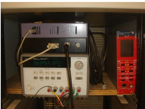
Figure 6-6 There're detector, high voltage power supply and low voltage power supply in the top section of the cabinet
