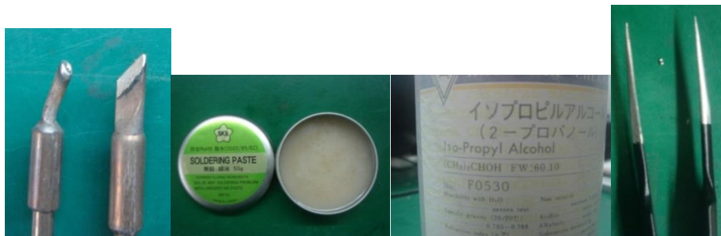
Figure 3-11 Soldering tools: soldering iron, soldering paste, isopropyl alcohol, tweezers (from left to right)
