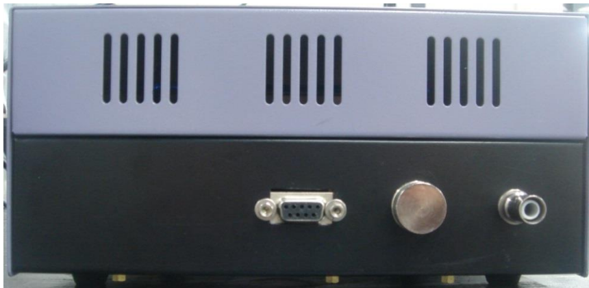
Figure 4-4 Back of the case with connectors
