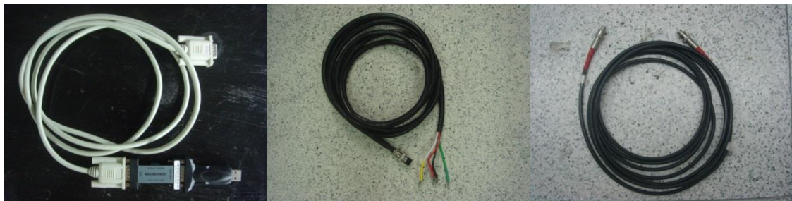
Figure 4-5 Cables for BGO system: RS232, LV power, HV power (from left to right)
