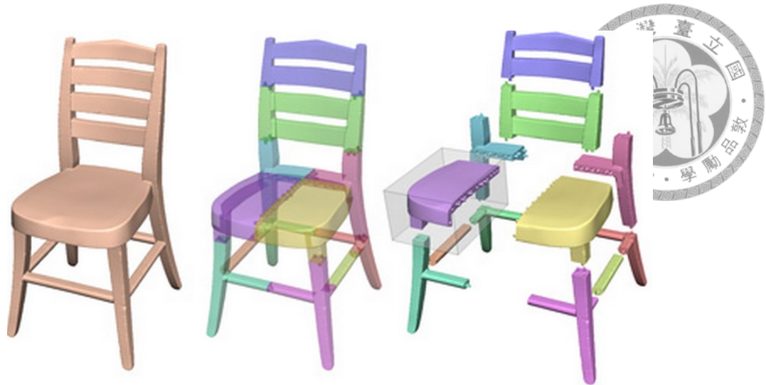
Figure 3.3: Large-scale construction using 3D printer by "Chopper: Partitioning Models into 3D-Printable Parts".
