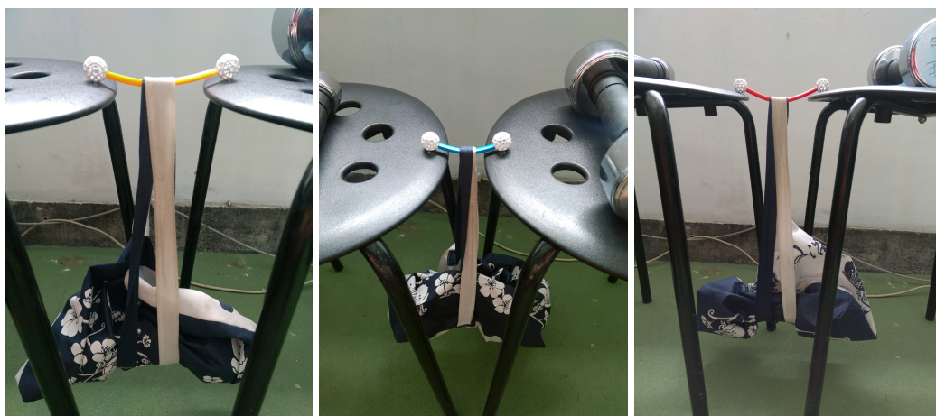
Figure 8.4: The extreme situation for three types of struts. The color of the middle part of struts become lighter, and we stop adding force when it happens. Weight of dumbbell for yellow strut is 3 kilogram; Weight of dumbbell for blue strut is 5 kilogram; Weight of dumbbell for red strut is 4 kilogram.
