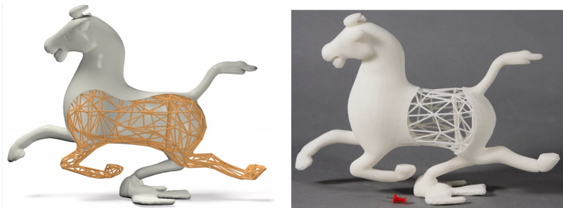
Figure 3.1: 3D printer acceleration of construction by "Cost-effective Printing of 3D Objects with Skin-Frame Structures".
