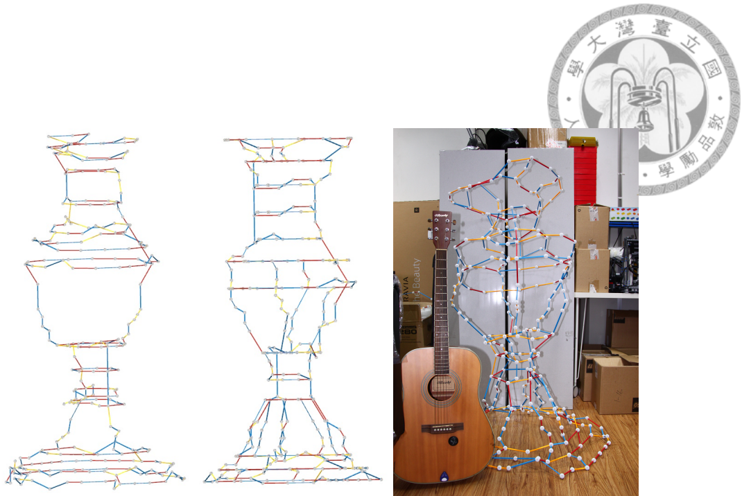
Figure 6.7: Results of vase. Left one is the base result, middle one is the refine result, and the right one is the real model constructed with Zometool.
