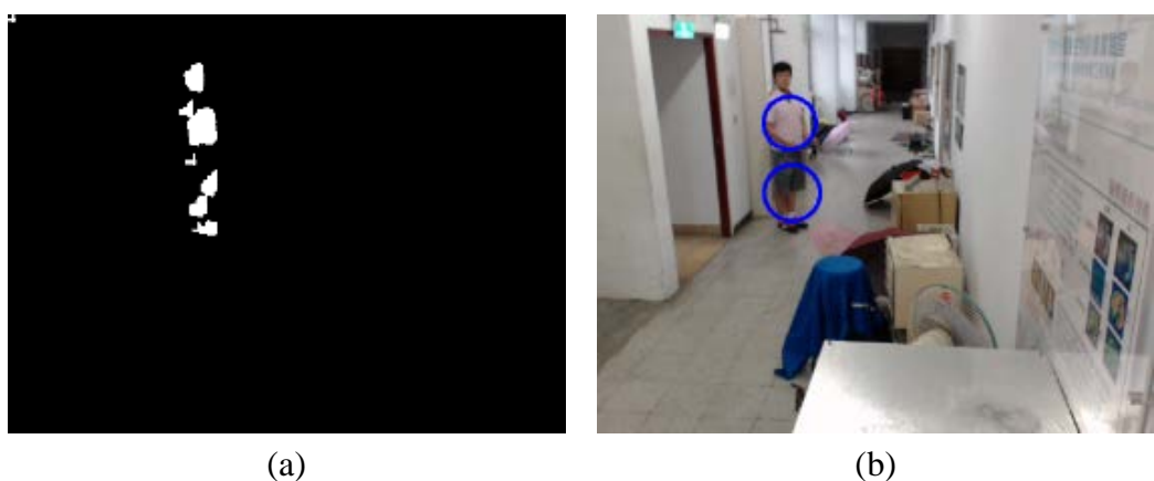
Figure 4-15 False alarm demonstration of the SOD algorithm. (a) The result of the detection. (b) The RGB version of (a)
