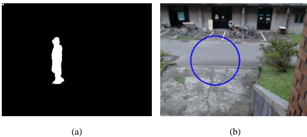
Figure 3-17 False alarm effect on fast self-tuning algorithm. (a) False alarm caused by a static interference source while using fast self-tuning background subtraction algorithm.
