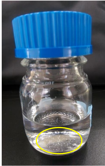
Figure 7 White particles collected from the solution contacting with lead pipe-stainless steel fitting connection.
