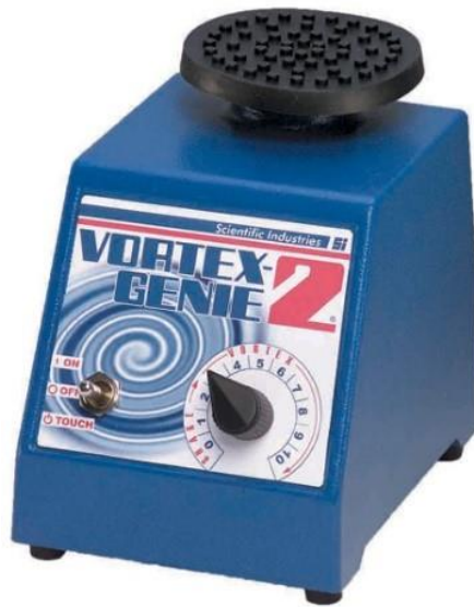
圖 3-13 震盪機(VORTEX-GENIE2 S5001, ZYMO RESEARCH)
