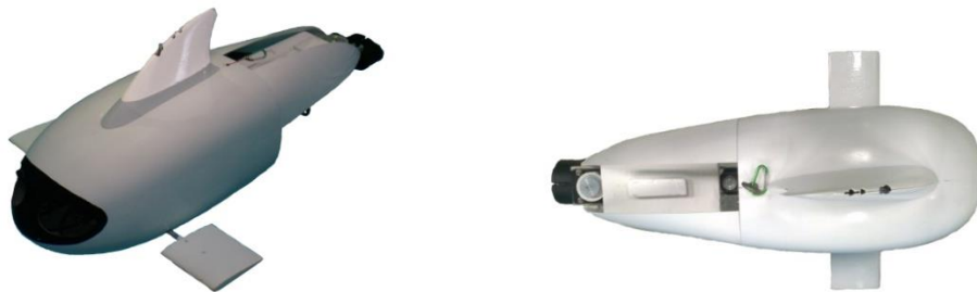
Figure 1.1 AUV pictured from the side and top with horizontal fins and a rotatable propeller.
