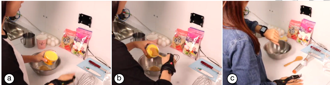
Figure 3.8: Logging daily activities on everyday things. (a) A user logs the procedure of cooking by (b) performing the tasks using the tagged object, and shares the logs with other users. (c) While another user drops the same tagged object, the system prompts the next step through the smartwatch display.
