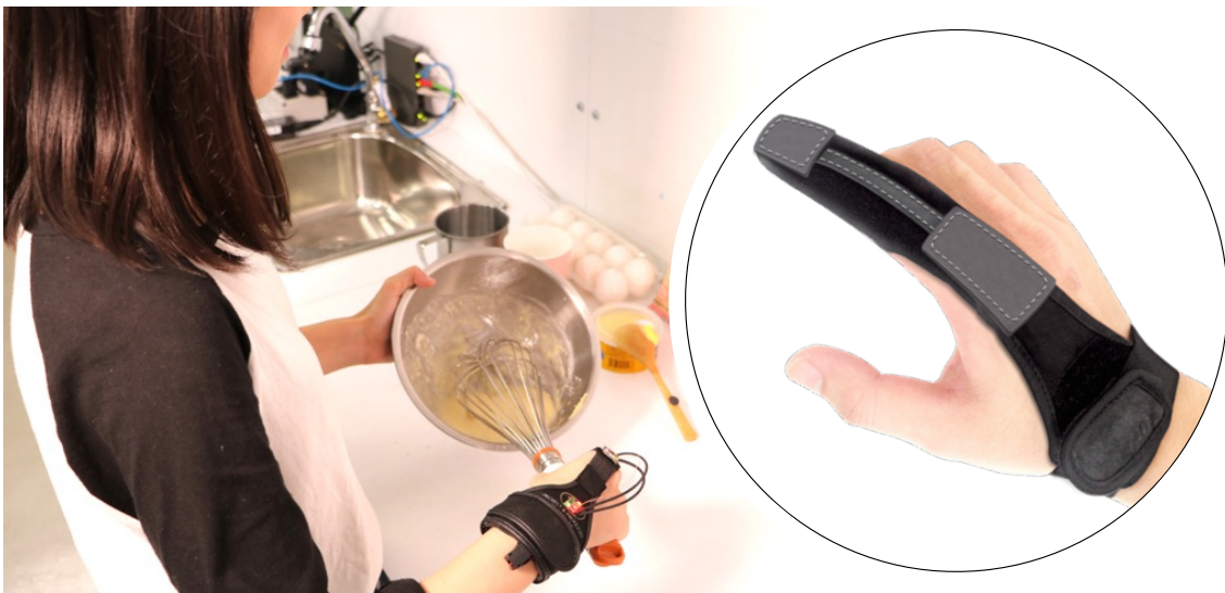
Figure 1.1: MidasTouch is a finger-worn device for sensing gestural input on everyday objects.
