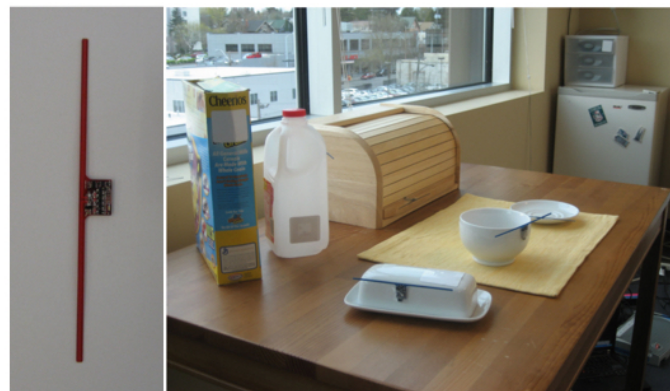
Figure 2.7: Related Works left: Wireless Identification and Sensing Platform (WISP) right: Tagged WISP on everyday objects to sense indoor activity
