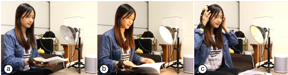
Figure 3.7: Connecting everyday things and smart things. (a) When a user opens the book, the lamp (b) turns the light on simultaneously. (c) When the user wears the headphone, the speaker mutes.
