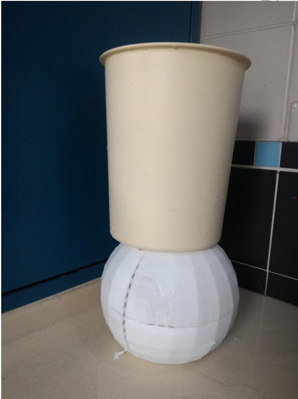
Figure 5.8: In the shell parts with connectors case, after we filled water into the bucket, the model deformed immediately and kept the shape still.
