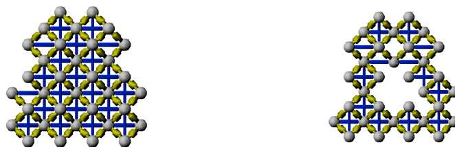
Figure 4.5: Eliminate unnecessary tetrahedrons (a) Fill out the entire volume. (b) Leave only a layer.
