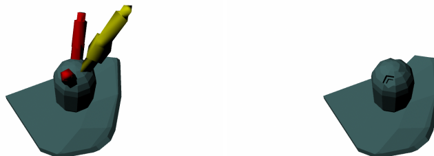
Figure 4.15: Connector. (a) Create a columnar body inside the segment. (b) Do Boolean difference to create slots to let zometool insert.
