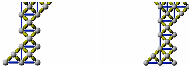
Figure 4.6: Avoid articulation points (a) Structure with articulation points. (b) Fill up tetrahedrons.
