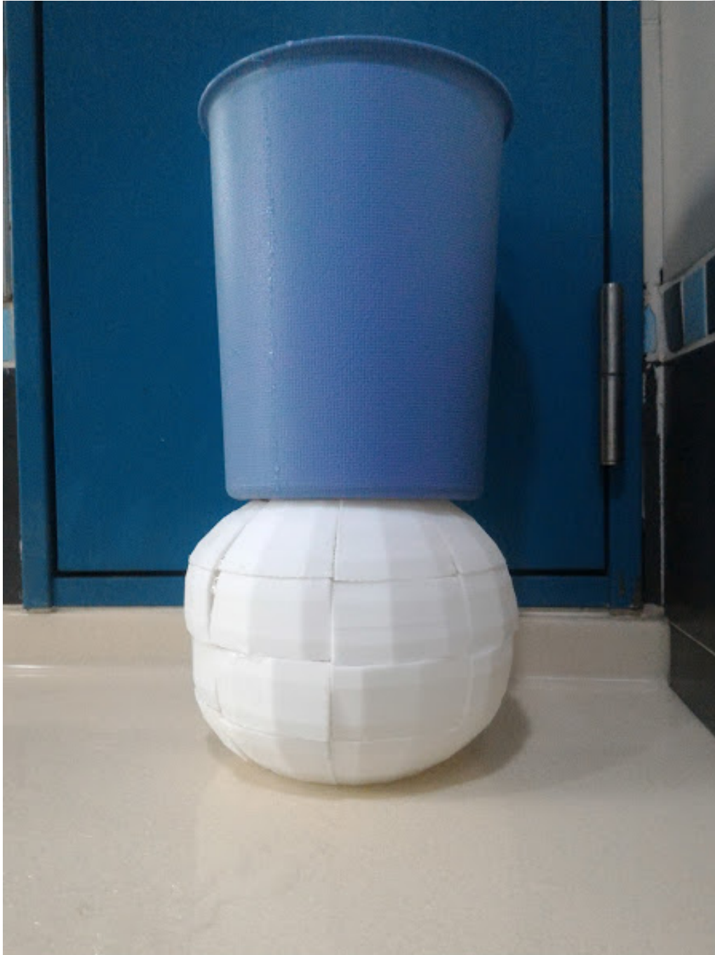
Figure 5.6: in shell parts with glue case, the seams would get bigger slowly after the water filled in the bucket.
