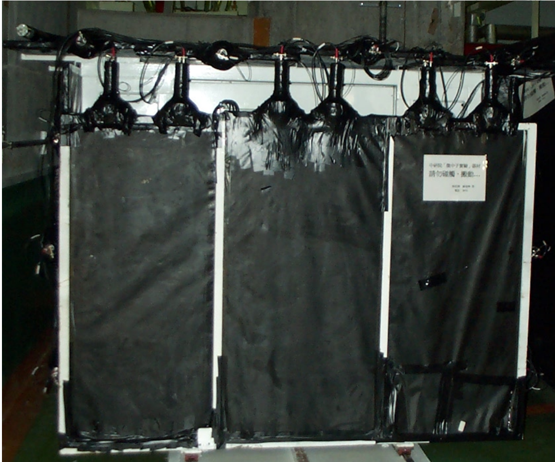
Figure 2.4: Photograph of the plastic scintillators (the black panels) at the front side and their attached PMTs on upper ends.
