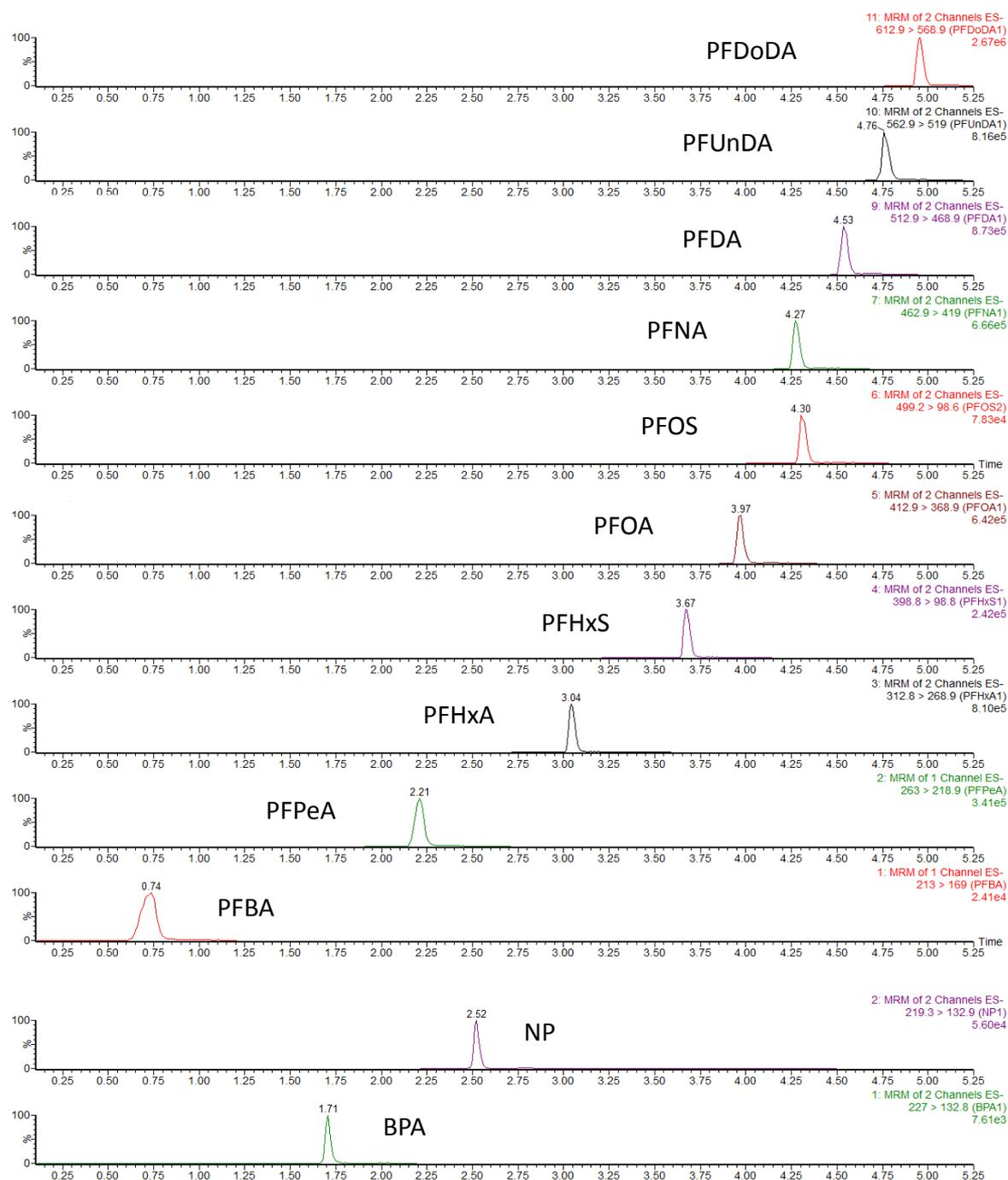
Figure 1. Chromatograms of 10 PFASs, NP, and BPA in MeOH (500 ng/mL, injection 4  $\mu$ L)
