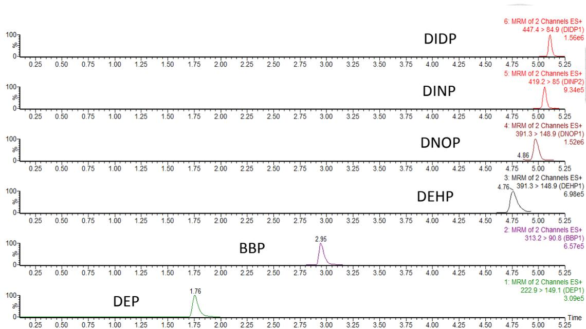
Figure 2. Chromatograms of six phthalate esters in MeOH (500 ng/mL, injection 4  $\mu$ L)
