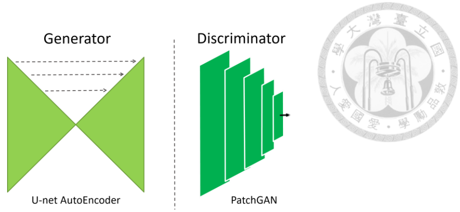
Fig. 3.8 Architecture of image-to-image Generative Adversarial Network [15].
