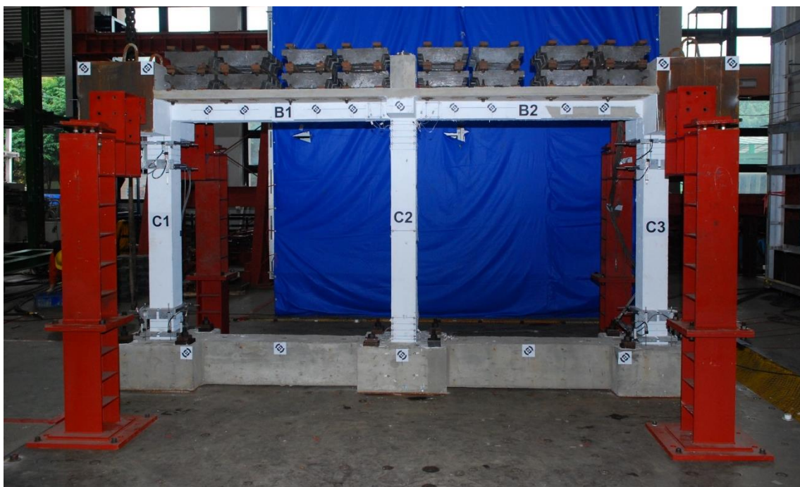
Figure 2-8 One-story two-bay reinforced concrete frame
