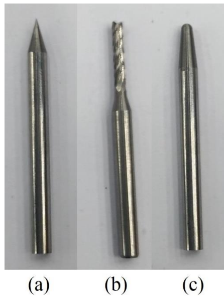
Figure 5.2-1 The three different carving tools. Left to right : (a) The cone drill. (b) The twist drill. (c) The round drill.
