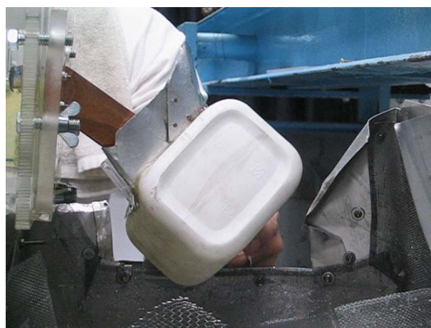
Figure 1.7 The method that measured the flow discharge directly using a customized funnel, which intercepted the flow and guided the mixture of flow to a bucket to measurements for 1–3 seconds.
