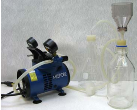
Figure 4. The 0.2- \mu\text{m} cellulose acetate filter (ADVANTEC) and a chemical duty vacuum pump (Millipore, MODE: WP6111560, 80-100psi).
