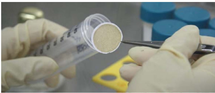
Figure 5. The 0.2- \mu\text{m} cellulose acetate filter was used to collect microbes (ADVANTEC).
