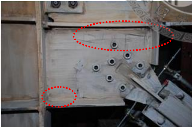
(e) 試體三上端接合板降伏 (+0.02 rad)
