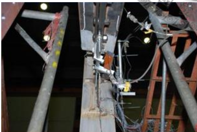
(e) 試體四上端接合板無面外變形(側視) (-0.02 rad)
