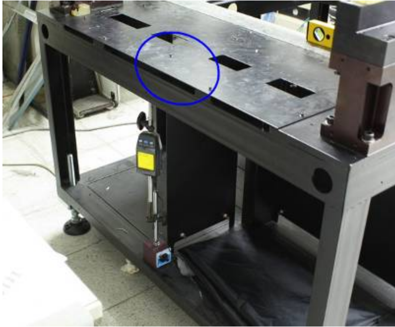
Figure 3-7 Static deformation experiment set up
