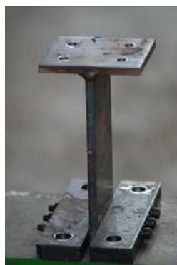
Figure 4-17: Close view of the bolting connection of the connecting plates.
