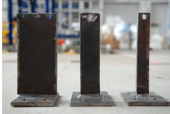
Figure 4-16: Connecting plates installed in the bracing system of the 1/4-scale 6-story steel building structure (left: B3; middle: B2; right: B1).
