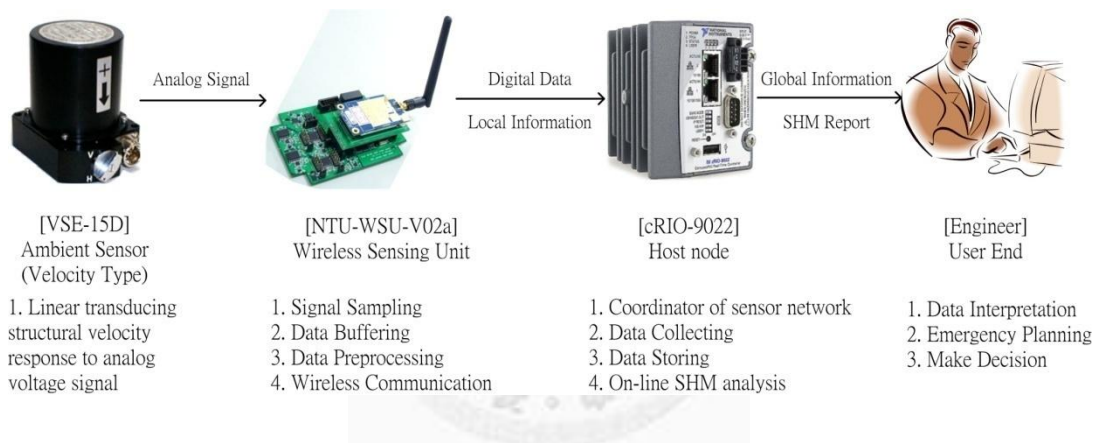
Figure 2.2: Function overview of Smart Sensing System.
