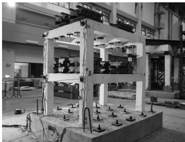
Figure 3.9: (a) Photo of the specimen A1F frame, (b) Photo of the specimen P1F frame, (c) Photo of the 2-story RC frame structure.
