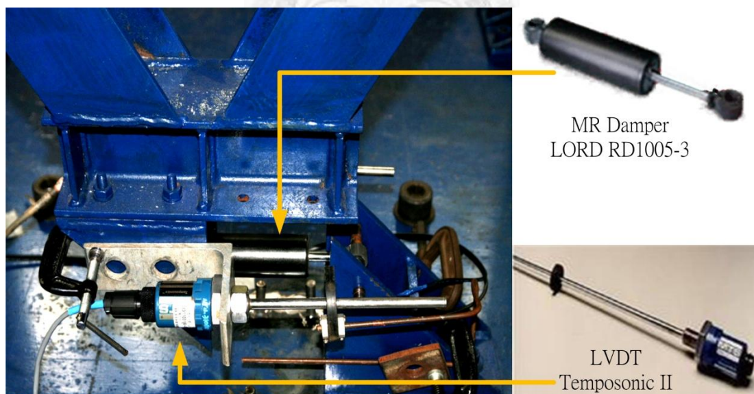
Figure 4.2: The detail view on the bracing of 6-story structure
