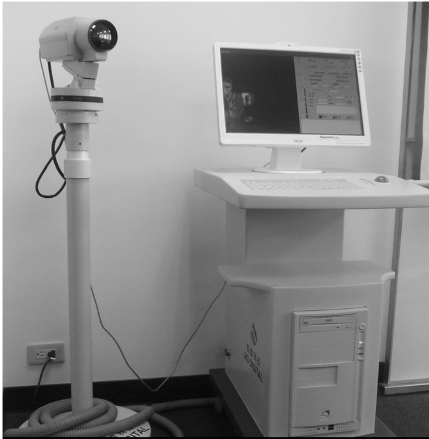
Figure 2. The thermographic machine. The computer for image storage and processing (right) and the thermographic camera (left) are shown (ATIR-M301 Thermographic Imaging System, Associated Technology Corporation, Chongqing, Sichuan, PROC). (The figure was offered by Yuh-Ming Wu, Department of Biomedical Engineering, National Taiwan University Hospital.)
