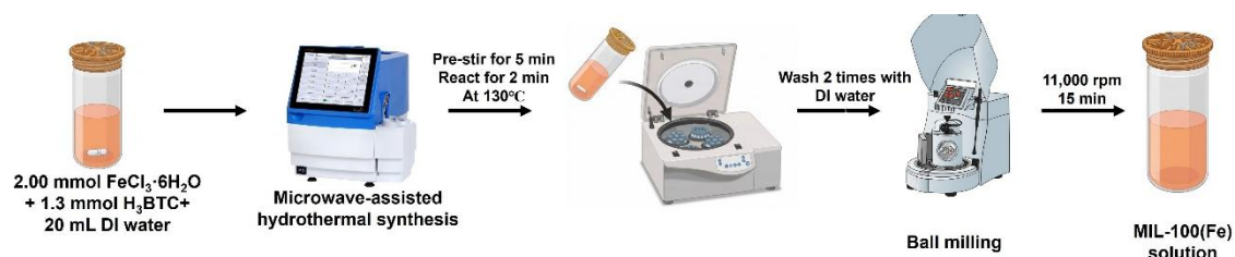
Figure 4.1 Schematic illustration of the microwave-assisted synthesis and ball-milling process of MIL-100(Fe).
