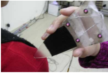
Figure 2.2.7 Using the stylus to locate and digitize the desired anatomic landmarks relative to the rigid body of sensor.
