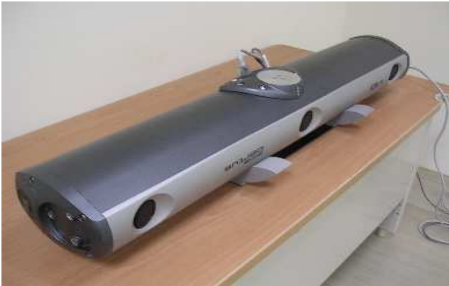
Figure 2.2.5 The position sensor used in this experiment was OPTOTRAK CERTUS from Northern Digital Inc., Canada. Each position sensor was embedded with three cameras to sense three-dimensional positions of LED markers.
