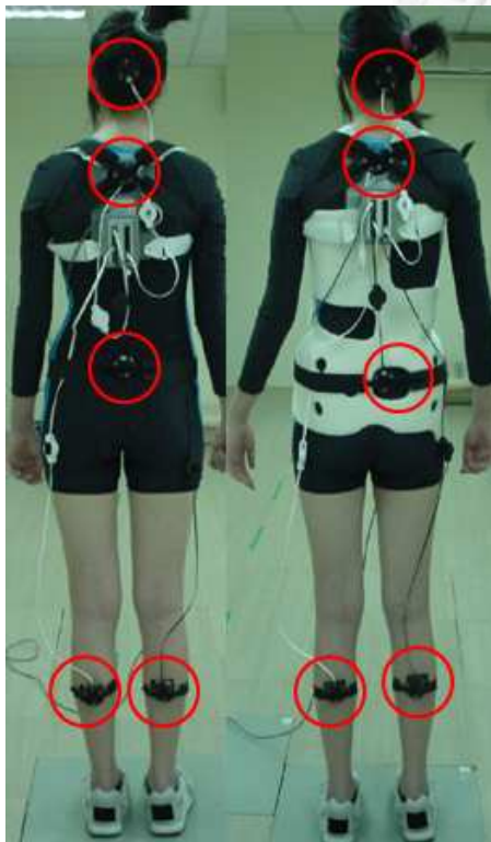
Figure 2.2.6 Five rigid bodies were placed at selected locations. Each rigid body with three LED markers on it generated a local coordinate system of each segment.
