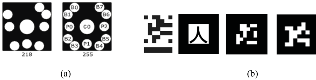
Figure 2-16: The vision-based tags (a) domino tag (b) The examples of the markers from CyberCode, ARToolkit, ARToolkit Plus and ARTag (from L to R)
