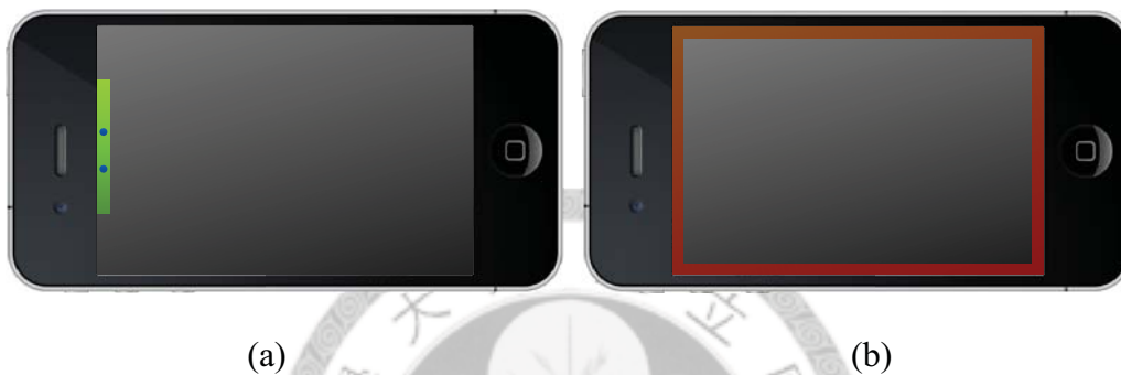
Figure 4-9: two modes of Detector object. (a) Fixed-position mode: clip-on gadget has to be attached to specific positions. (b) Dynamic-position mode: clip-on gadget can be attached to arbitrary positions on the edge.
