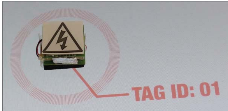
Figure 3-11: Animated progress ring appears around the tangible object while the frequency tag is being identified
