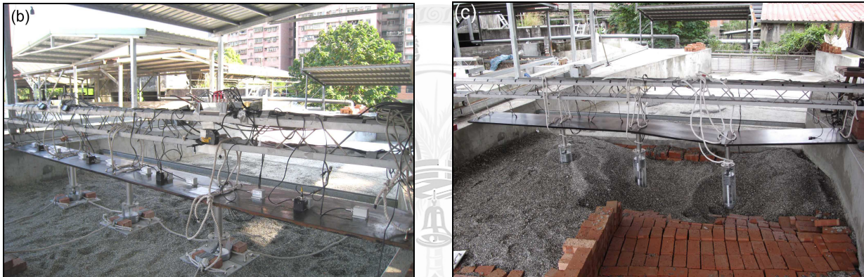
Figure 7-28 (a) Bridge configuration and sensors location (b) Field setup of the bridge (c) After concluded the scouring experiment
