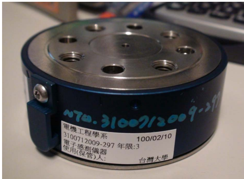
Fig. 15 The 6-axis force sensor “IFS-67M25T50- M40BS”
