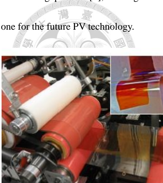
Figure 1.3 Roll-to-roll manufacturing process of polymer photovoltaics [3]
