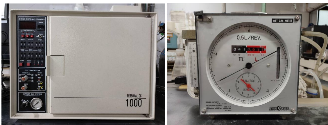
Figure 3-7 GC (left) and wet test gas meter (right) for gas analysis
