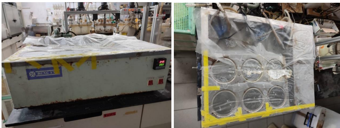
Figure 3-4 Water bath's front view with its thermostat (left) and top view with the water pumps (right)
