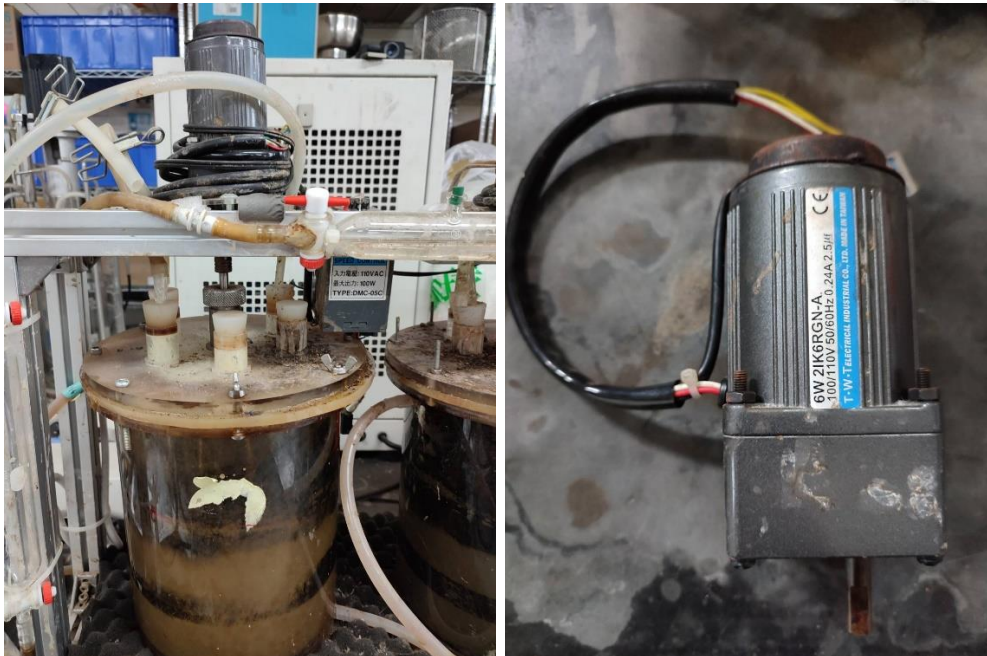
Figure 3-5 One of the reactor that was used for batch operation (left) and motor that was used to drive the mixer (right)
