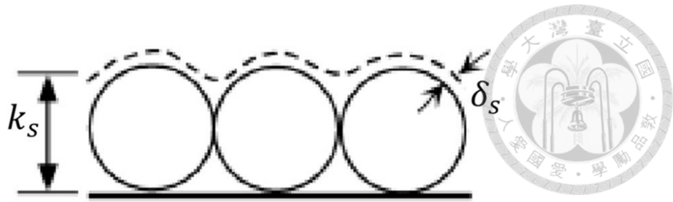
Figure 4.2 Turbulent flow under the condition of the rough bed boundary (modified by MIT note).
