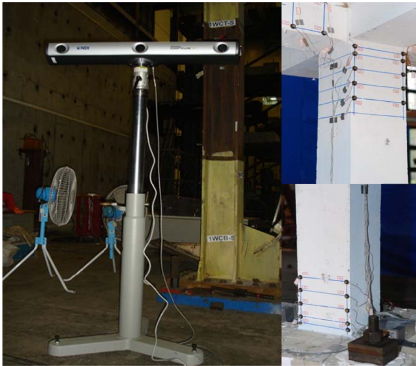
Figure 3-5 Optical sensing system in the shake table test
