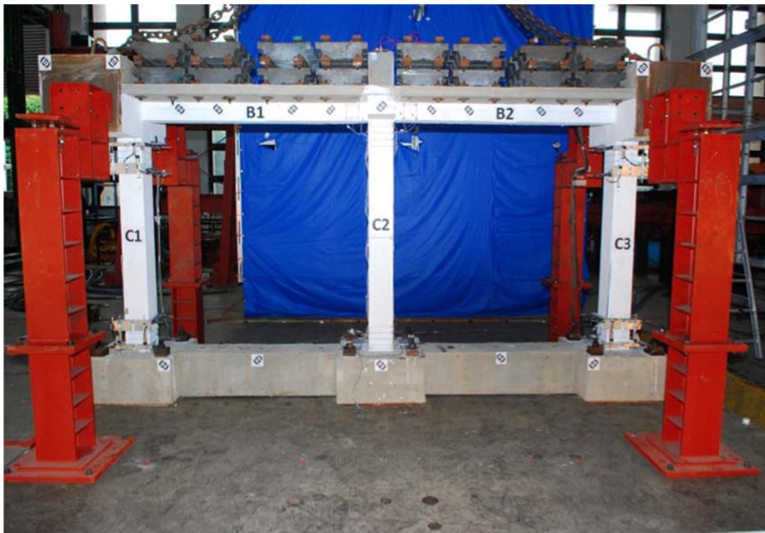
Figure 3-1 Specimen of one-story two-bay RC frame
