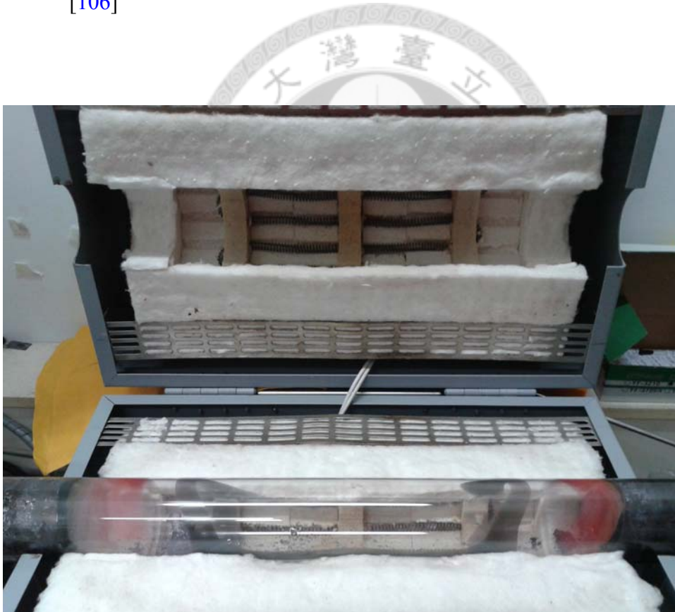
Fig. 3-5 Vacuum quartz furnace for the CIS selenisation
