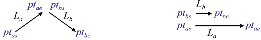
(a) d(p_{as}, p_{ae}) = d(p_{bs}, p_{be}) , t_{ae} - t_{as} = t_{be} - t_{bs} . (b) d(p_{as}, p_{ae}) = 3d(p_{bs}, p_{be}) , t_{ae} - t_{as} = 3(t_{be} - t_{bs}) .
