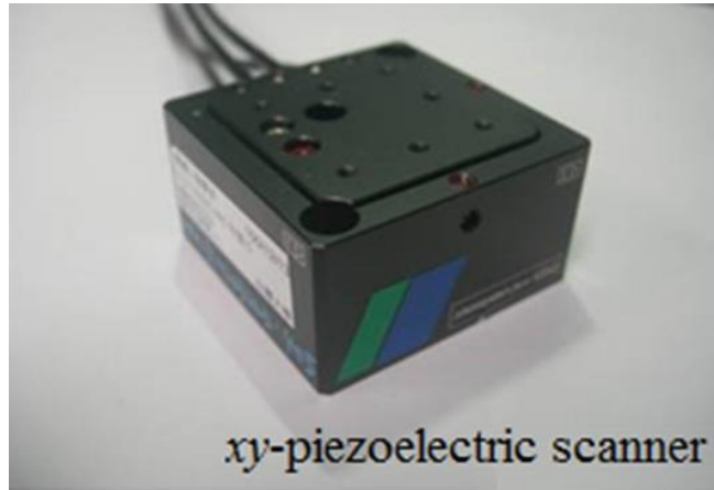
Fig. 3-8 Realistic photograph of the piezoelectric xy -scanner
