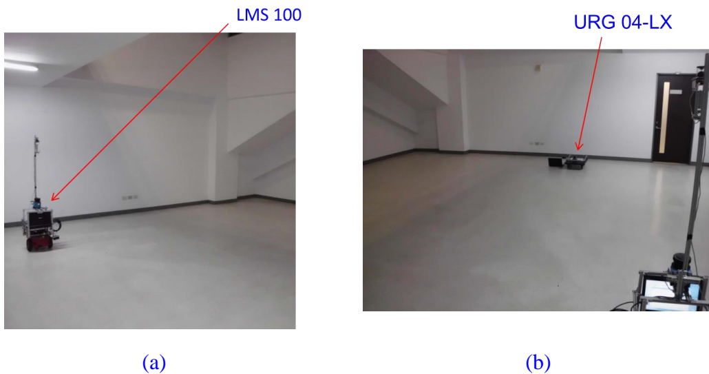
Figure 5.25 The Experimental Scene in Ming-Da Building 4F (a) The LRF LMS100 mounts on the Pioneer 3-DX for localization (b) The URG 04-LX measurement as a ground truth
